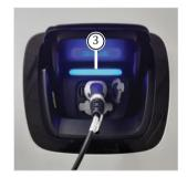
If the charging process has started correctly, LED "3" flashes blue. Check this to make sure.
