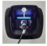
Take the charging cable from the charge point and insert it into the vehicle. Lock the car with the Mobility Card (hold card up to the checkpoint).
