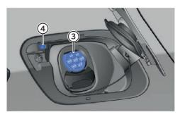
Take the charge cable from the charging station and plug it into the vehicle charging socket "3". Lock the car with the Mobility card (hold card at checkpoint).
