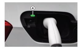
If the charging process has been started correctly, LED indicator "4" at the charging socket flashes green. Check this to make sure.
