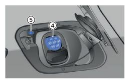
Take the charge cable from the charging station and plug it into the vehicle charging socket "4". Lock the car with the Mobility card (hold card at checkpoint). Charging starts automatically, or if necessary you can activate the charging station using the "Home charging card". Check this on the LED "5" at the charging socket. This has to be flashing green if the car is being charged properly.
