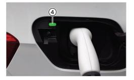
If the charging process has been started correctly, LED indicator "4" at the charging socket flashes green. Check this to make sure.
