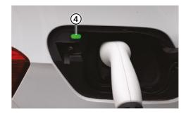
If the charging process has been started correctly, LED indicator "4" at the charging socket will flash green. Check this to make sure.
