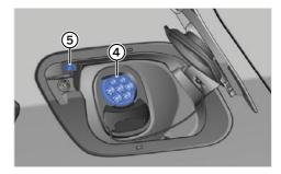
Take the charge cable from the charging station and plug it into the vehicle charging socket "4". If available, hold the charging card, located in the card holder in the glove box, up to the charging point to start the charging process. Lock the car with the Mobility Card (hold card at checkpoint).
