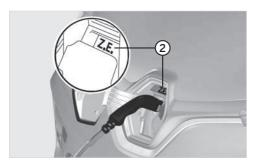
If the charging process has been started correctly, the "Z.E." symbol flashes blue (2). Check this to make sure.
