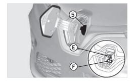
Take the charge cable from the charging station and plug it into the vehicle charging socket "E". Charging starts automatically, or if necessary you can activate the charging station using the "Home charging card". Check this on the "Z.E" symbol at the charging socket. This has to be flashing blue if the car is being charged properly. Lock the car with the Mobility card (hold card at checkpoint).
