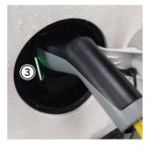
If the charging process has been started correctly, charge indicator "3" at the charging socket flashes green. Check this to make sure.
