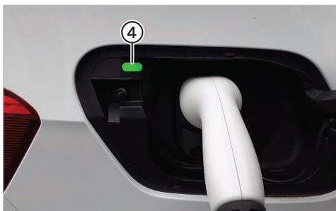
If the charging process has been started correctly, LED indicator "A" at the charging socket flashes green. Check this to make sure.
