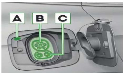
Take the charge cable from the charging station and plug it into the vehicle charging socket “B”. If available, hold the “Home” charging card, located in the card holder in the glove box, up to the charging point to start the charging process. Lock the car with the Mobility card (hold card at checkpoint). Charging starts automatically. Check this on the LED “A” at the charging socket. This has to be flashing green if the car is being charged properly.
