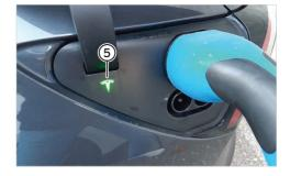
Take the charge cable from the charging station and plug into the upper vehicle charging socket. Lock the car with the Mobility card (hold card at checkpoint).
