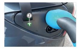
If the charging process has been started correctly, LED "2" flashes green.
