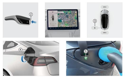
Take the charge cable from the charging station and plug into the upper vehicle charging socket. Lock the car with the Mobility card (hold card at checkpoint). Charging starts automatically, or if necessary you can activate the charging station using the "Home charging card". Check this on the LED "5" at the charging socket. This has to be flashing green if the car is being charged properly.
