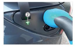
If the charging process has been started correctly, LED "2" flashes green. Check this to make sure.
