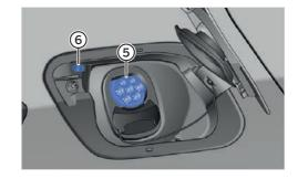
Take the charge cable from the charging station and plug it into the vehicle charging socket "5". Lock the car with the Mobility card (hold card at checkpoint).
